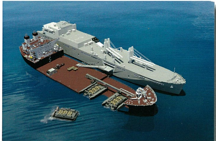
Conducting vehicle transfer operations from an LMSR to LCAC for transport ashore
