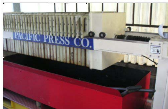
The Filter Press "squeezes" excess water
