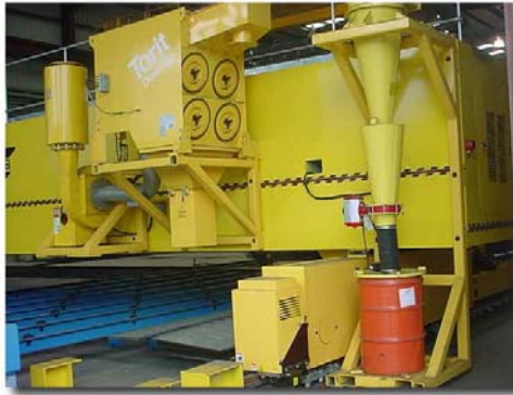
Abrasive blast waste collection for recycling at the Block Assembly Line.
