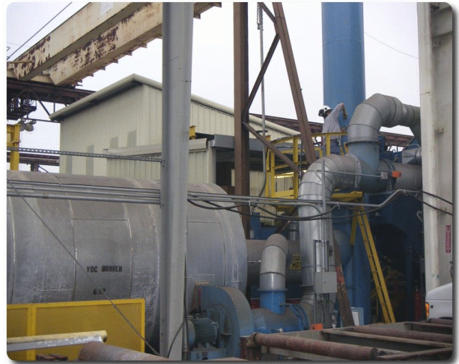
APCD Air Pollution Chemist Ian Morris sets up equipment to monitor the concentration of VOCs at the Primeline #2 thermal oxidizer exhaust.
