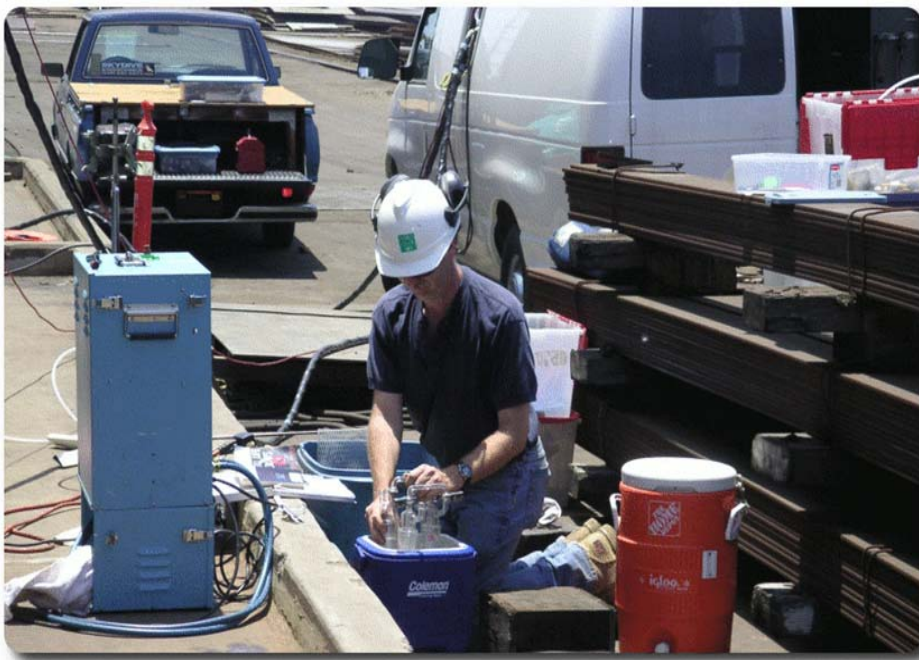
APCD Air Pollution Chemist Ian Morris takes samples of the exhaust gas from Primeline #1 oxidizer to determine water content.
