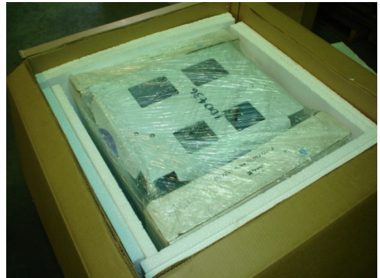
See above for a correct example of proper cushioning and internal spacing inside of a box or crate.
